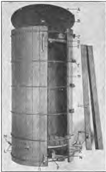
FIG. 30.—Quick vinegar generator, staves removed showing interior. (Hydraulic Press Mfg. Co.)
